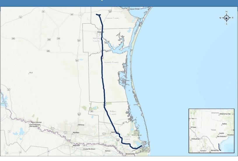
The Bay Runner Pipeline is an approximately 145-mile intrastate pipeline designed to transport up to 2.64 billion cubic feet per day of natural gas from the Agua Dulce, Texas supply area to a terminus near Port Isabel, Texas, providing direct access to global markets and consumers.
