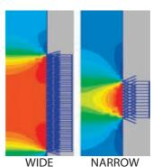
Computational pressure distribution inside the limb when applying the NARROW HemaClear® or the WIDE Pneumatic Tourniquet
