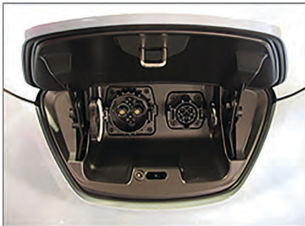
FIGURE 3 Photo shows a standard J1772 inlet on the right for use with Level 1 and Level 2 chargers; and a CHAdeMO inlet on the left. Photo from U.S. Dept. of Energy Energy, Efficiency and Renewable Energy Website: ( http://www.afdc.energy.gov/fuels/electricity_infrastructure.html ).
