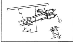
1. Adjusting nut (brake cable)
