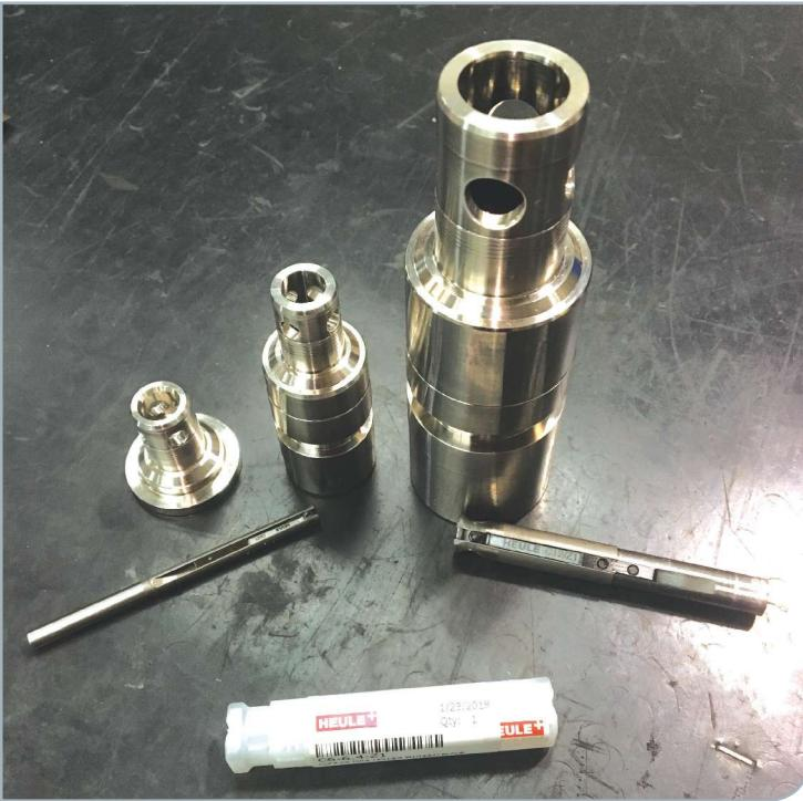
∴ The Cofa C-series tooling is for 1/4-inch, 1/2-inch and 3/4-inch holes. This automated deburring tool is specifically designed for front and back deburring using CNC machinery.
