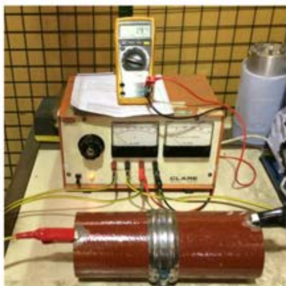
Electrical Continuity Testing
