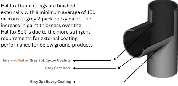
The Halifax Drain fittings are coated internally with either red or grey 2-pack epoxy to a minimum average thickness of 150 microns. This paint has also been subjected to the same stringent testing regime as the other components of the system. These tests include a 350-hour salt-spray test, a 30-day waste water test at 23°C and a series of dimensional checks
