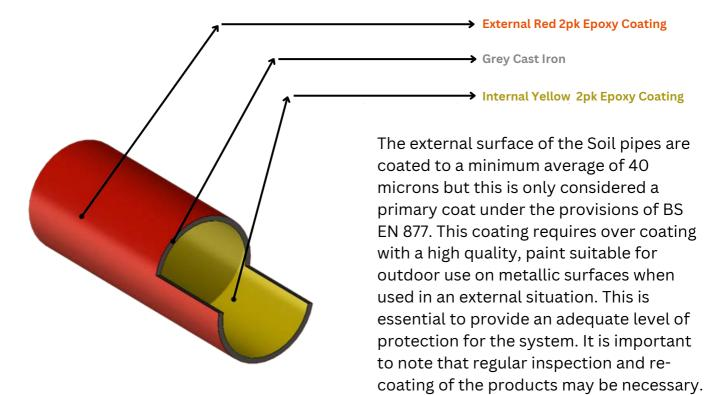
The external surface of the Soil pipes are coated to a minimum average of 40 microns but this is only considered a primary coat under the provisions of BS EN 877. This coating requires over coating with a high quality, paint suitable for outdoor use on metallic surfaces when used in an external situation. This is essential to provide an adequate level of protection for the system. It is important to note that regular inspection and re-coating of the products may be necessary.
