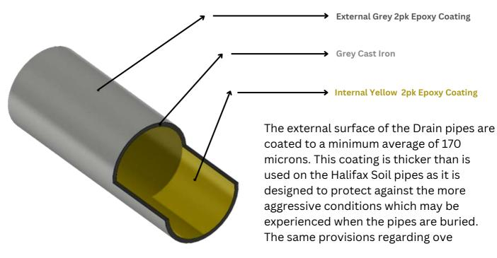
The internal surface has a minimum average coating thickness of 130 microns. This enables the Halifax Drain pipes to withstand a variety of tests designed to reproduce the conditions that the products will encounter in their working life. This includes a 30-day waste water test at 23°C, a 30-day chemical resistance test at both PH 2 and PH 12 and a 1500 cycles water temperature test between 15°C and 93°C.
