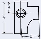
**"87.5° SINGLE RADIUS CURVE BRANCH WITH 2" BSPT BOSS ON RIGHT"**
