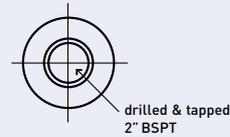
**BLANK ENDS DRILLED & TAPPED 2"**
