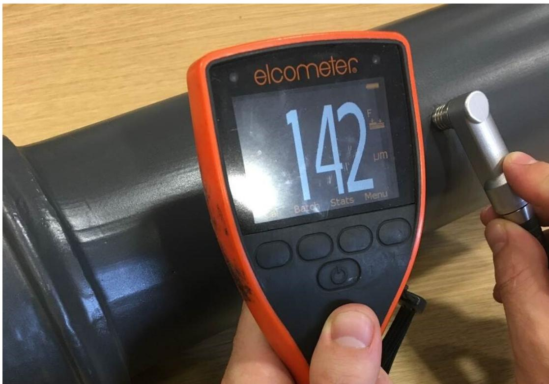
Dry film thickness (DFT) is a non-destructive coating thickness measurement, using techniques which do not damage the coating or the substrate such as magnetic, magnetic induction and eddy current thickness measurement methods.
