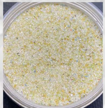
SchabelTech RCF - 55 Recycled ~ 40/70 Mesh
