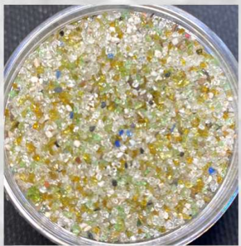
SchabelTech RCF - 590 Recycled ~ 20/40 Mesh
