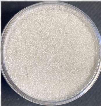
SchabelTech WQZ #551 White Rounded ~ 20/40 Mesh
