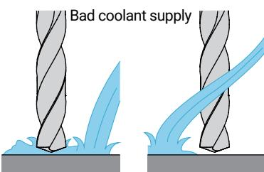
Three coolant pipes should be directly towards the drill tip when it's possible.
