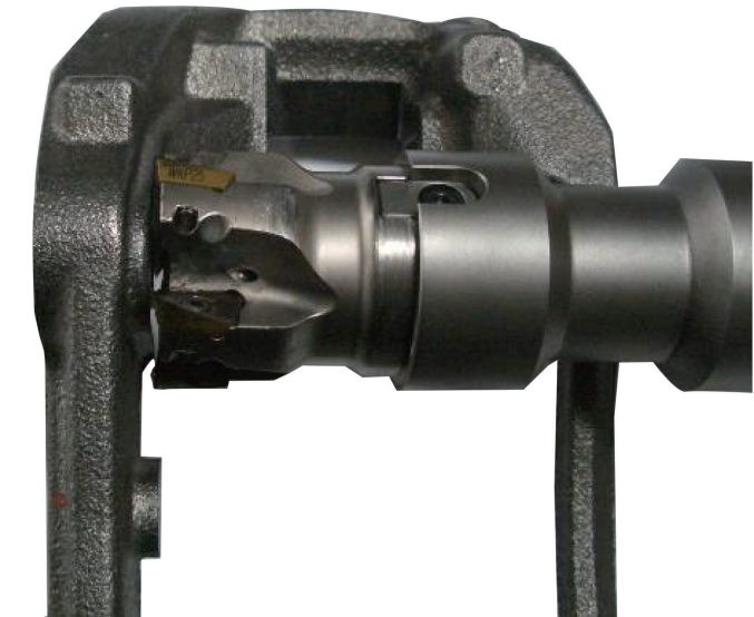
Application: Side milling Solution: Achteck AP series
