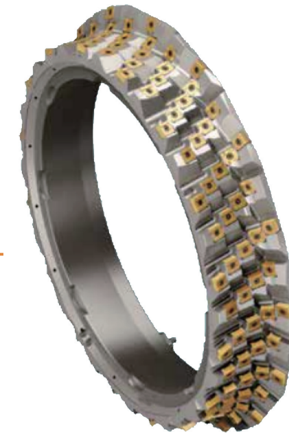
Profile milling for rail re-shaping
