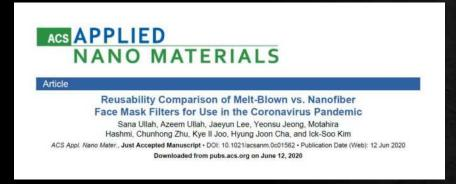
When MB filter was sprayed with ethanol and reused, the filtration efficiency was reduced by up to 64%. On the other hand, the nanofiber filter retained almost the same efficiency as the first time even after 10 reuses. This difference is due to the decrease in static electricity in the filter after spraying. Unlike MB fibers, nanofibers are filtered according to the morphological characteristics and nano size spiracle of the surface, so efficiency is maintained after cleaning.
