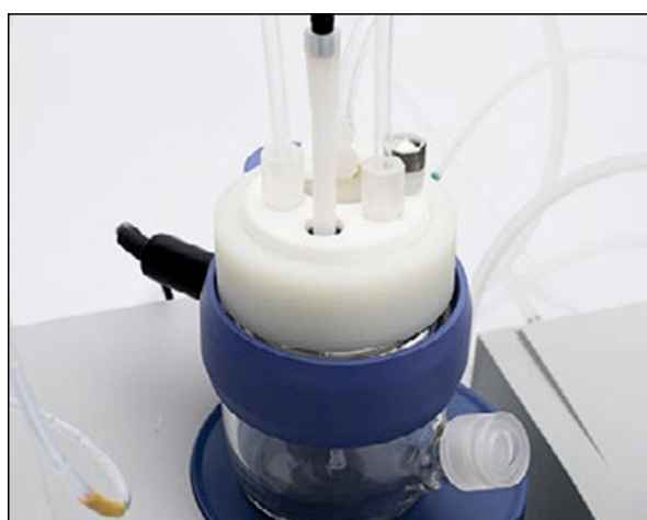
Sample titrate unit, Suitable for constant moisture samples
