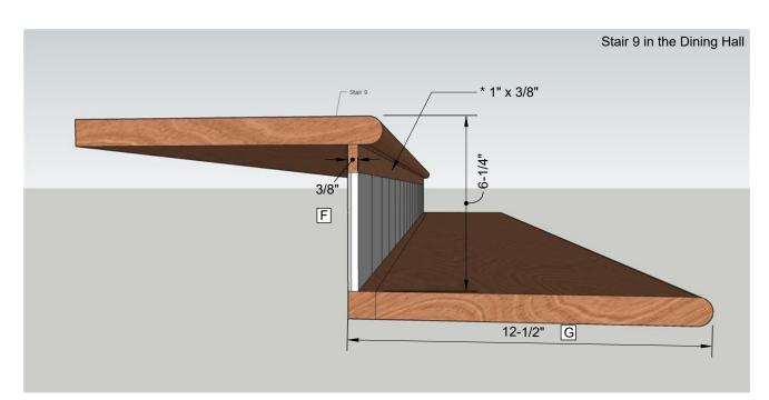
\* 100 LF of 2" white oak trim to go above riser tiles. Minimum width 3/8", maximum width 1/2" to maintain code variance. Rip cut to fit in place above tile and below bullnose of every riser, installing flush to sub-riser. Stain in place to match.
