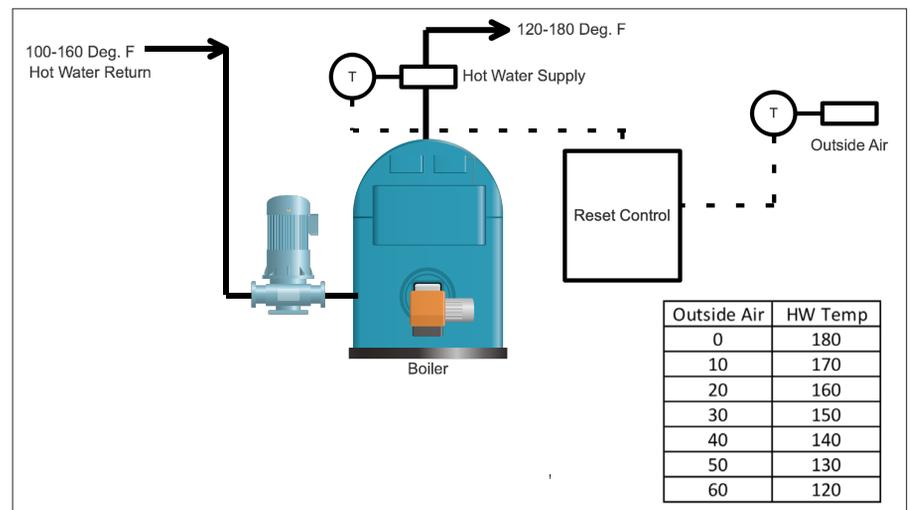
**Be careful using a reset control on a boiler not designed for low temperatures. It could cause flue gas condensation.**
