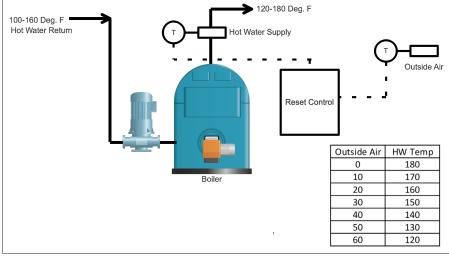
Be careful using a reset control on a boiler not designed for low temperatures. It could cause flue gas condensation. owner contacted the manufacturer of the boiler and asked what would cause the damage. After sending pictures of the internal damage and showing the reset control settings, the boiler manufacturer informed the owner the damage was caused by flue gas condensation.
