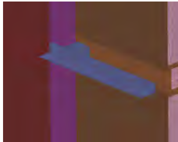
Fig. 3-8 Three-dimensional section of a standoff shelf angle supporting anchored masonry veneer
