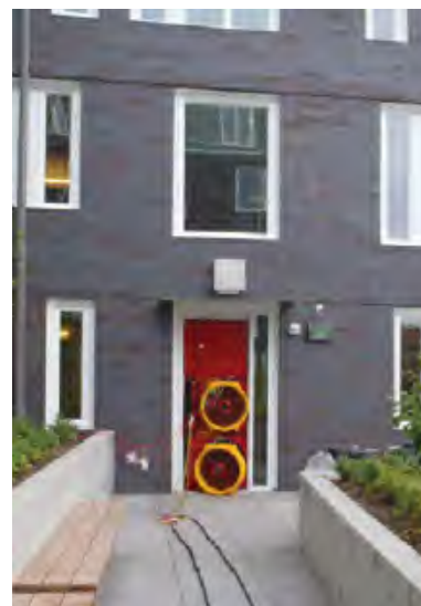
Fig. i-27 Blower door setup during whole-building air leakage testing of a building with an anchored masonry veneer above-grade wall system
