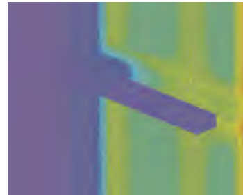
Fig. 3-9 Three-dimensional thermal image of the standoff shelf angle shown in Fig. 3-8
