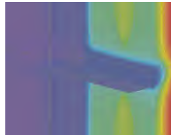
Fig. 3-7 Three-dimensional thermal image of the continuous floor line shelf angle shown in Fig. 3-7
