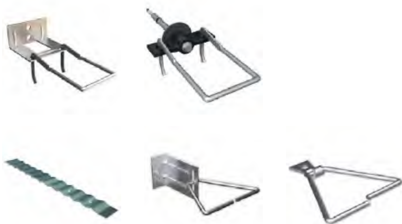
Fig. 3-15 Brick tie types. Top row, left to right: standard double eye and pintle plate tie, thermally optimized double eye and pintle screw tie. Bottom row, left to right: corrugated masonry tie, adjustable L-bracket, nonadjustable surface-mounted tie.
