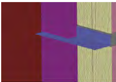
Fig. 2-10 Three-dimensional section of a continuous floor line shelf angle supporting anchored masonry veneer
