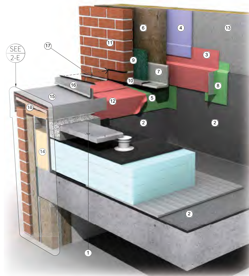
Saddle Flashing Cutaway Section
