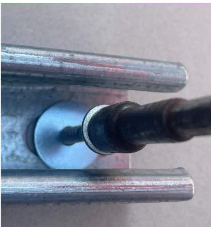
Tighten rail assembly at Spindle center-point recess using Feature-1 of the Spindle Spanner™
