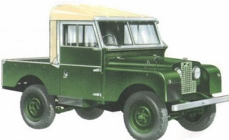
Above: The Land-Rover fitted with metal truck cab (available at extra cost), providing an all-enclosed, weather-proof driving compartment and leaving the rear section open for ease of loading or unloading.
