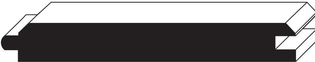
Tongue & Groove V-Joint SDW651 3/4" x 5-1/4"
