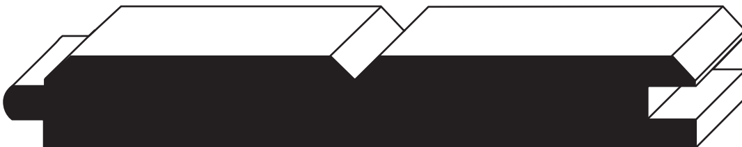
Tongue & Groove V-Joint / V-Center SDW652 3/4" x 5-1/4"
