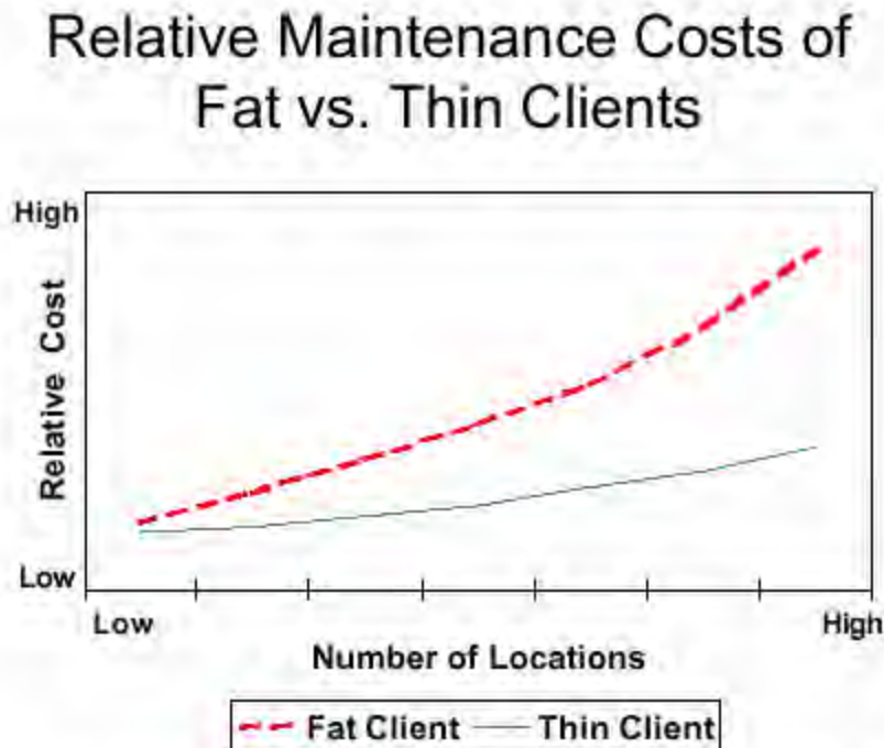
Figure 3 – Relative costs for maintaining fat vs. thin clients as the number of locations increases
