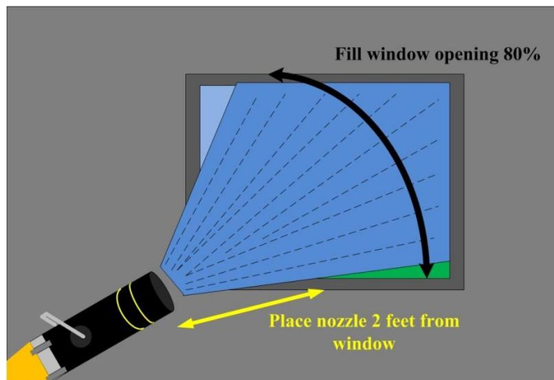
**Figure 6: Hydraulic ventilation.**
