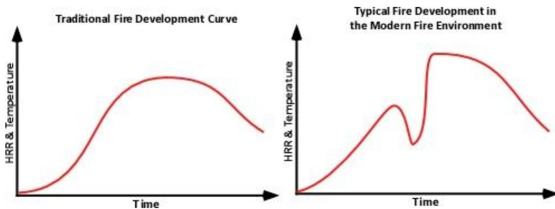
**Figure 3: Traditional vs. modern fire development curve.**
