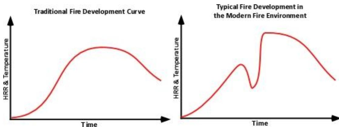
**Figure 3: Traditional vs. modern fire development curve.**
