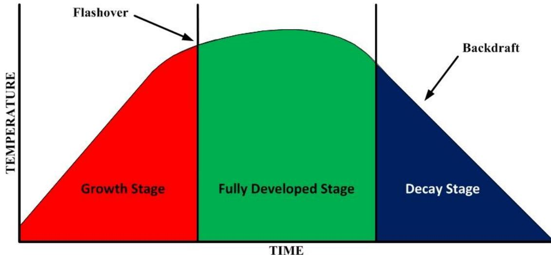
**Figure 5: The temperature curve and stages of fire.**
