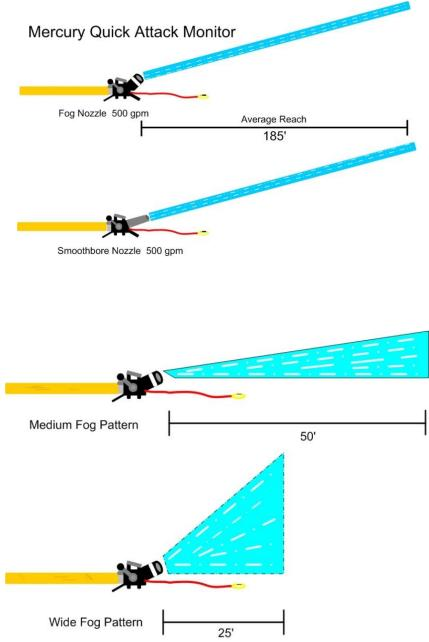
Figure 20: Ground monitor reach depends on the nozzle and pattern used.
