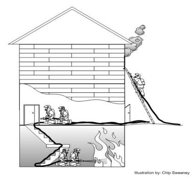
Figure 21: Hoseline placement for a basement fire in a single-family dwelling basement with no exterior entrance.
