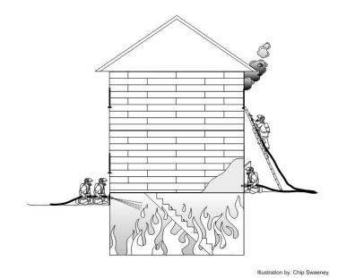
Figure 20: Hoseline placement for advanced basement fire conditions in a single-family dwelling basement with no exterior entrance.
