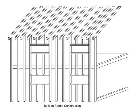
Figure 12: Graphic representation of balloon frame construction.
