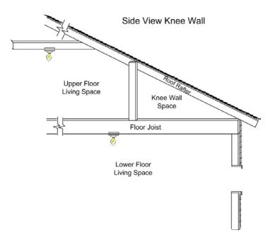
Figure 13: Cross section showing a knee wall.
