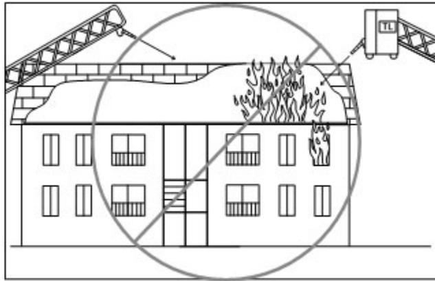
**Figure 92: Avoid having streams flow down onto the roof or through the fire area**
