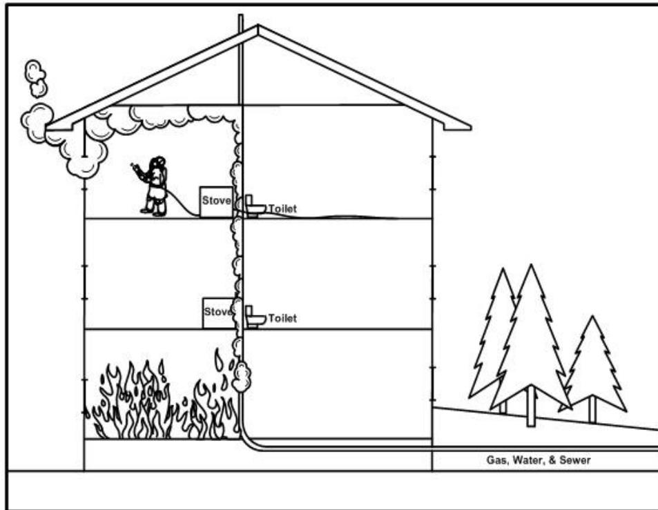
**Figure 87: Smoke and fire can travel in voids and utility shafts.**
