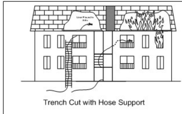
**Figure 94: Trench cut with hose support.**
