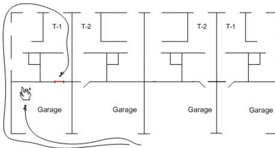
Figure 65: Fire in attached garage.
