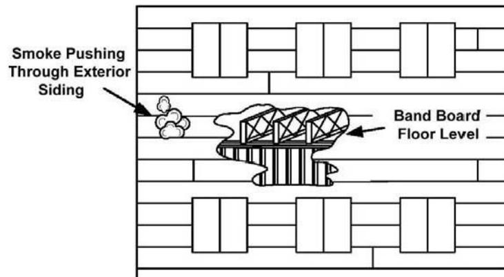
Figure 27: Smoke issuing from the band board area can indicate fire has breached the truss floor space.
