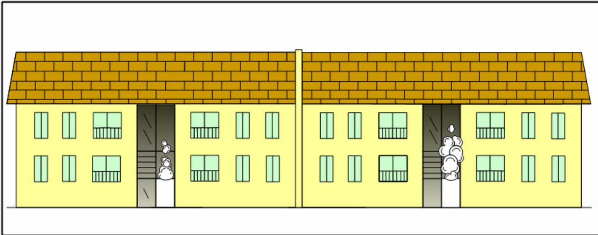
**Figure 59: Smoke showing from more than one stairwell is an indication of a basement/terrace-level fire.**
