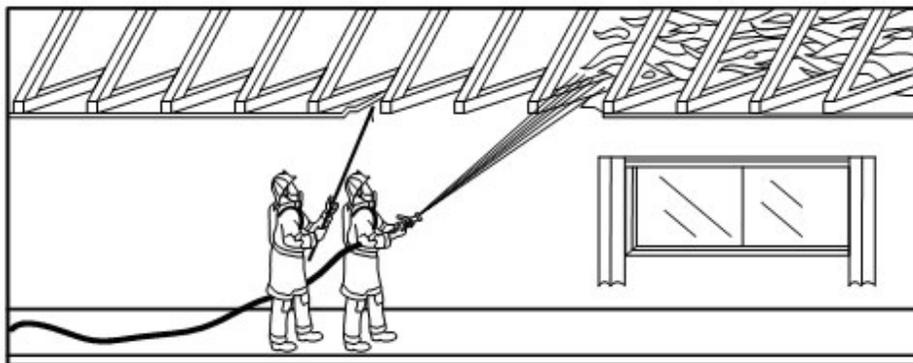
**Figure 69: Projecting a hose stream into an attic.**
