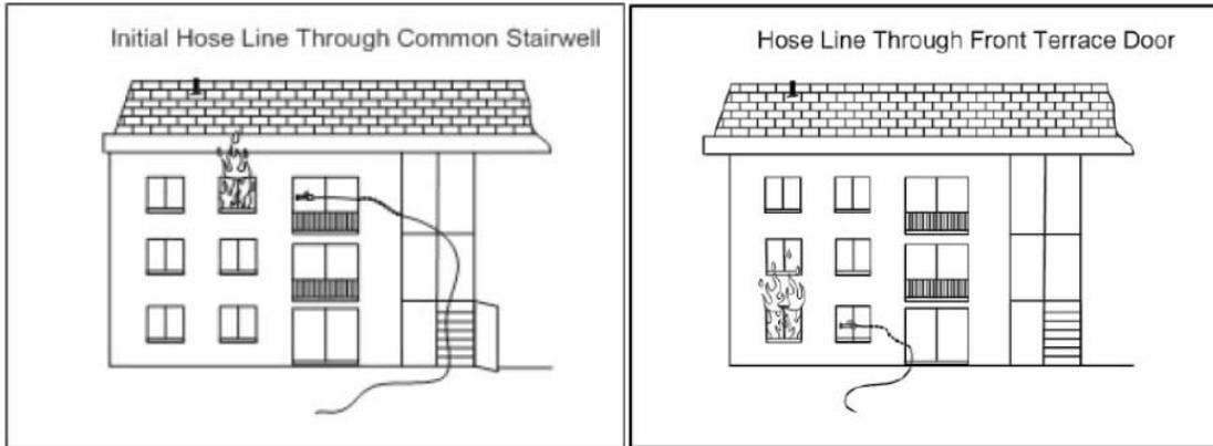
Figure 54: Common stairwell hoseline advance versus terrace-level advance.
