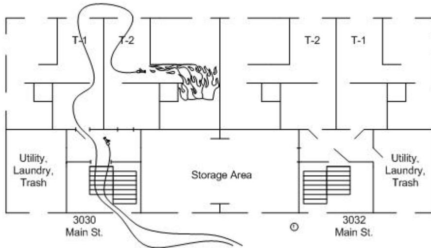
**Figure 61: Alternate terrace fire attack.**
