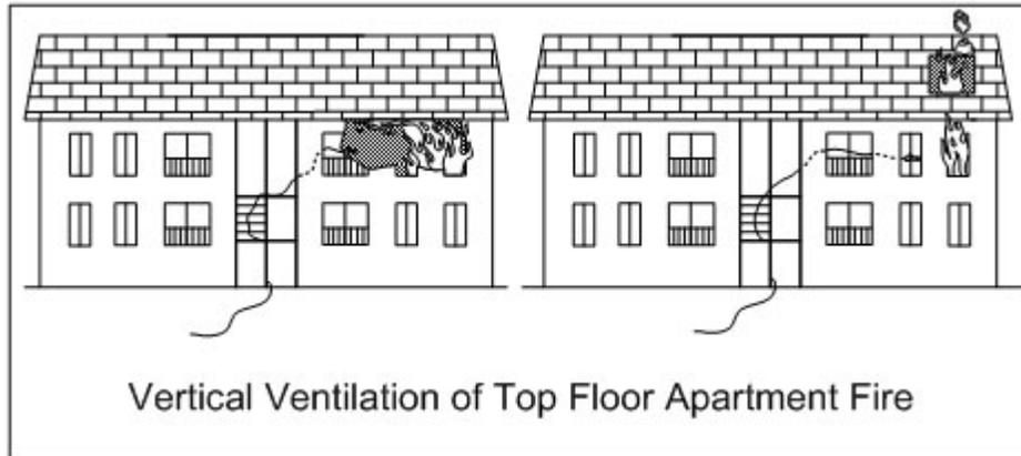
**Figure 82: Vertical ventilation of a top floor fire.**
