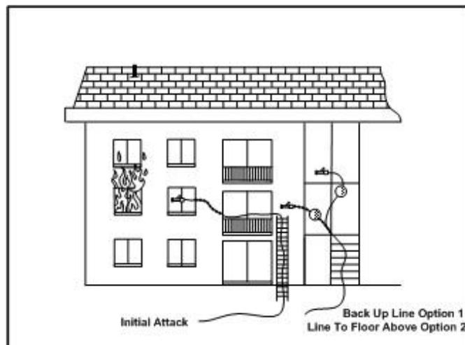
Figure 55: Example of the placement of a back-up line.
