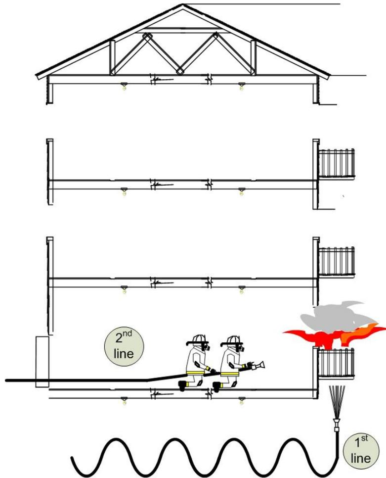
**Figure 37: Additional inside hoseline on exterior garden apartment fire.**
