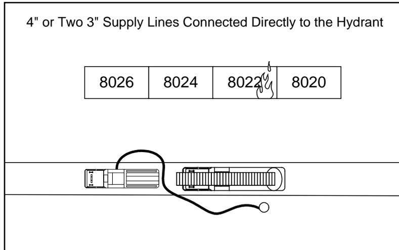
**Figure 43: Direct connection to hydrant.**
