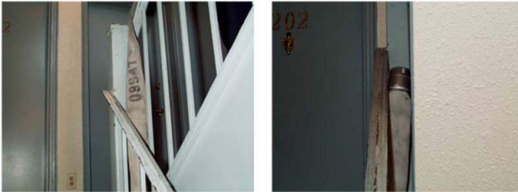
**Figure 48: Hose coupling jammed during hoseline advancement.**
