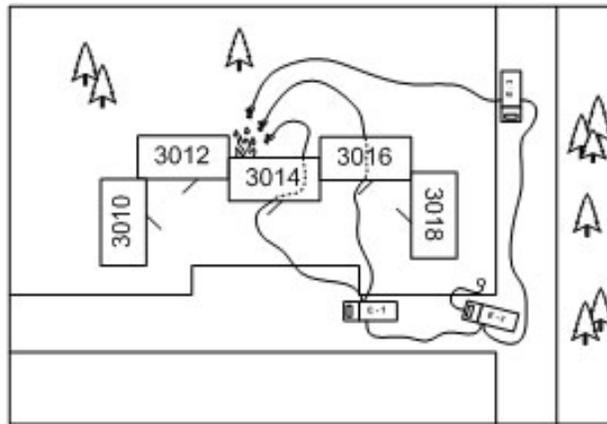
Figure 56: Options for hoselines to the rear of a structure.
