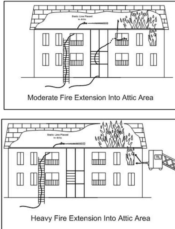
**Figure 68: Attacking attic fires.**
