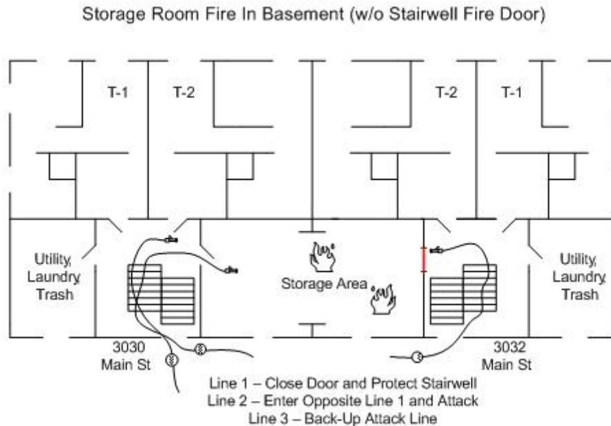
**Figure 64: Storage room fire in basement without stairwell fire door.**
