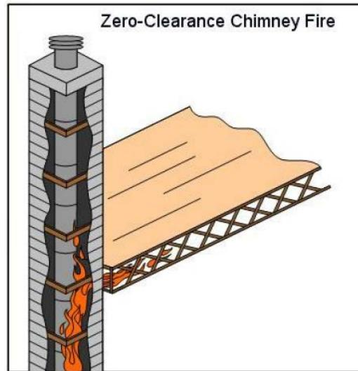
Figure 40: An example of fire spread between the floor and ceiling void space.
