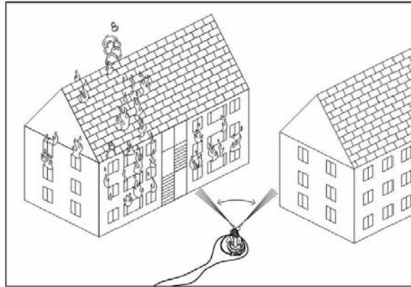
**Figure 57: Master stream protecting exposure.**
