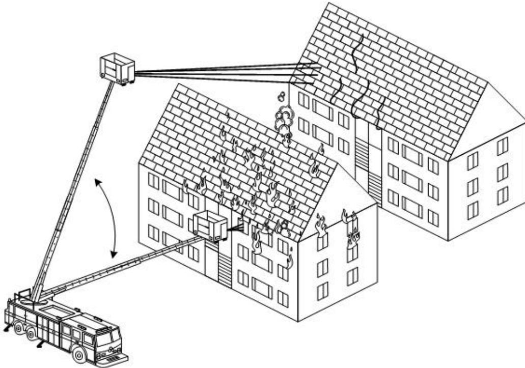
**Figure 97: Over the top to protect exposure.**
