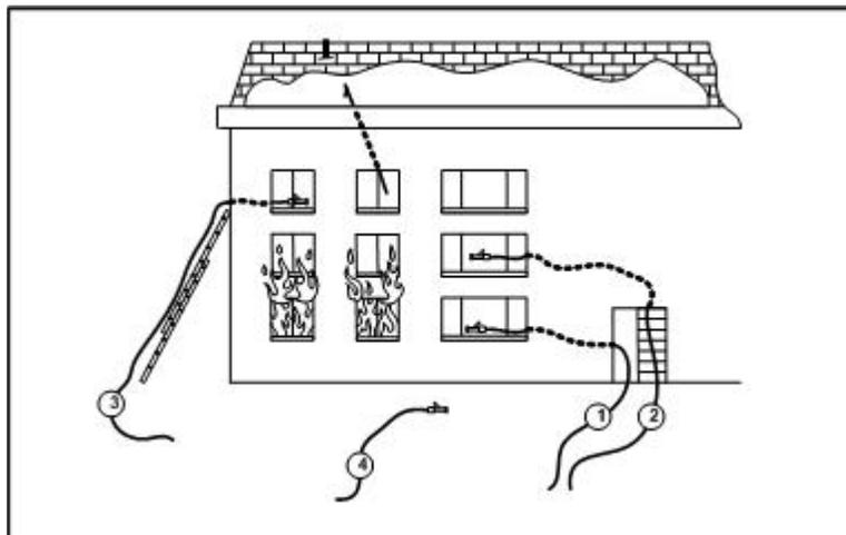
Figure 44: Typical initial hoseline deployment. Line 1 is the attack line. Line 2 is the back-up line/line above the fire. Line 3 is the top floor/attic line and Line 4 is the RIT/standby line.
