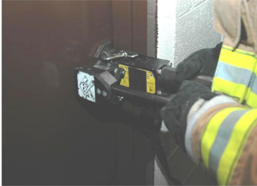
**Figure 79: Hydraulic forcible entry tool.**
