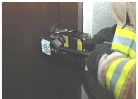
Figure 79: Hydraulic forcible entry tool.
