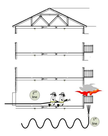
Figure 37: Additional inside hoseline on exterior garden apartment fire.
