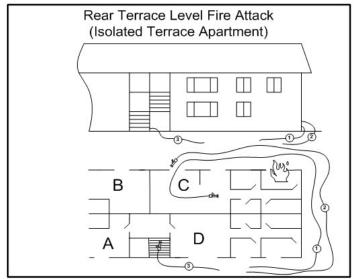
Figure 62: Rear terrace-level fire attack.
