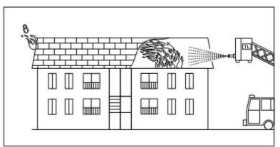
Figure 93: Wide fog pattern pushing fire across open attic.
