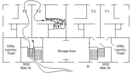
Figure 61: Alternate terrace fire attack.
