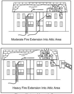
Figure 68: Attacking attic fires.
