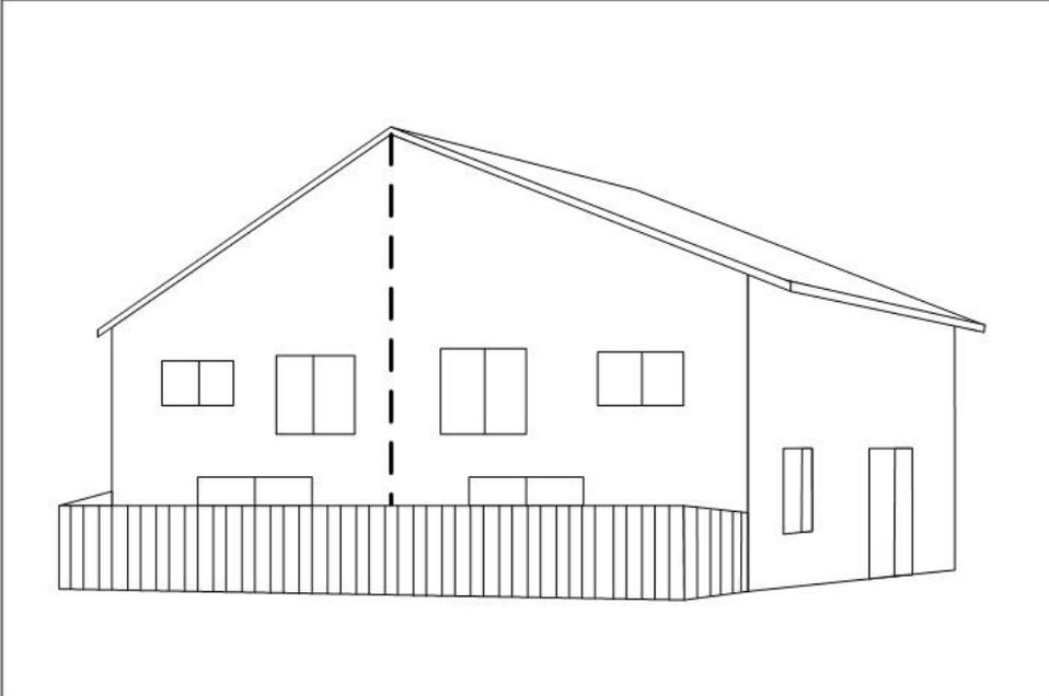
**Figure 2: A “back-to-back” is a townhouse consisting of two or more occupancies under one roof connected by the Side Charlie wall.**
