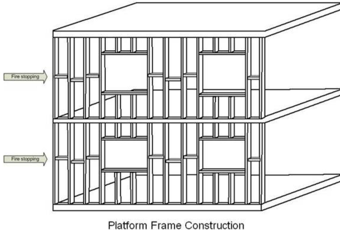
**Figure 9: Example of platform frame construction.**
