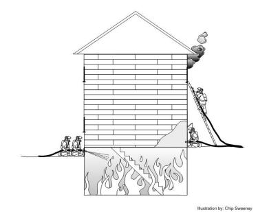
Figure 14: Hoseline placement for advanced basement fire conditions in a basement with no exterior entrance.
