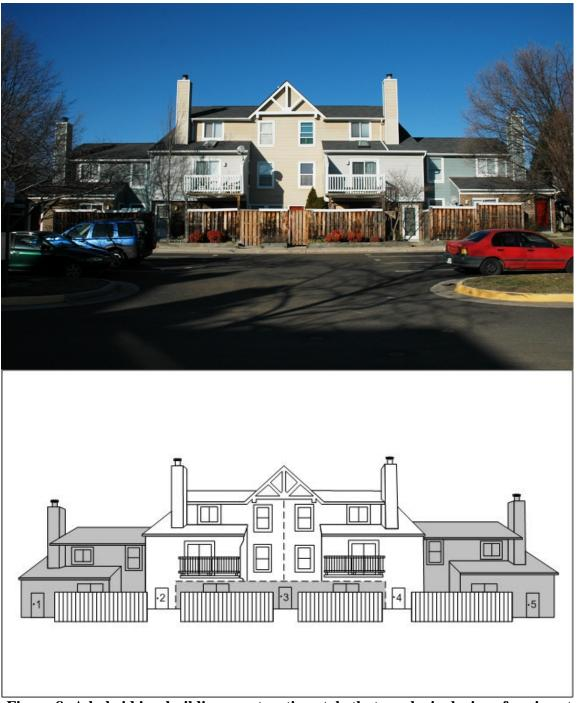
Figure 8: A hybrid is a building construction style that can be inclusive of various types of townhouse styles (piggyback, back-to-back, and over-under) under one roof. The figure shows the duplex from Side Charlie (top), and a diagram showing the five different occupancies (bottom).
