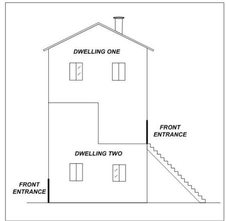
Figure 3: A piggyback townhouse consists of two stacked dwellings (one over the other), each with a separate address and entrance. These occupancies share a common floor separated by a fire wall on that floor. The figure shows the piggyback townhouse from Side Alpha (left upper), Side Charlie (right upper) and a cross-section diagram (lower).
