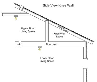
Figure 10: Cross section showing a knee wall.
