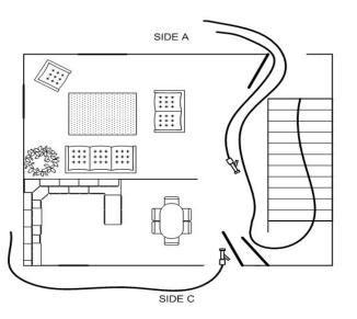
Figure 16: One of the doors (exterior or basement) needs to be completely removed to allow crews unimpeded access to the basement when entering from Side Charlie.
