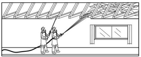
Figure 19: Projecting a hose stream into an attic.
