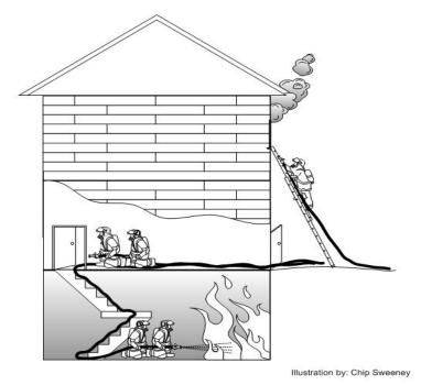
Figure 15: Hoseline placement for a basement fire in a basement with no exterior entrance.
