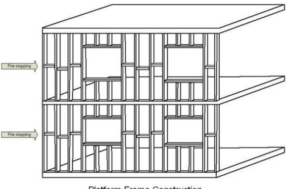
Platform Frame Construction Figure 9: Example of platform frame construction.
