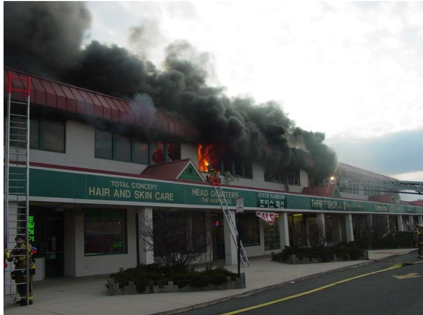
Figure 3. Horizontal fire extension in absence of firewalls.
