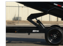
SCISSOR LIFT WITH POWERFUL CYLINDER
