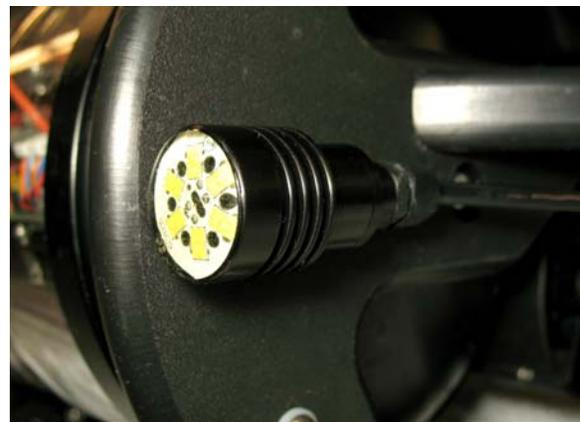
Image of a SeaBotix external 1080 lumen LED light.
