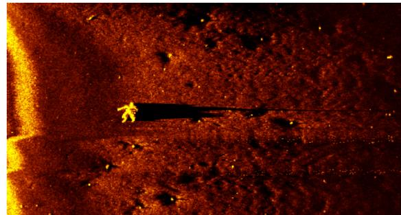
Victim's body imaged using a Marine Sonics Technology Centurion with a 900KH tow-fish in 40 m (131 ft) of water.
