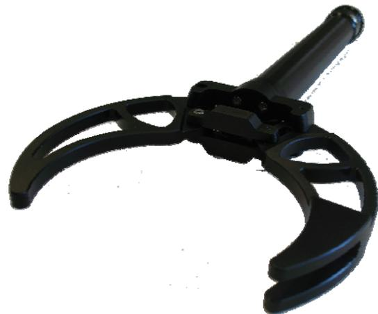
SeaBotix Large Interlocking Jaws with a 11.5 cm (4.5 in) opening (above).
