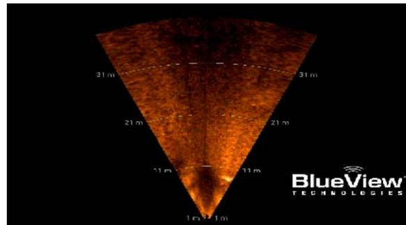
Three images approaching a drowning victim's body using a BlueView P450E multibeam sonar with a range set to 41 m (135 ft.).
