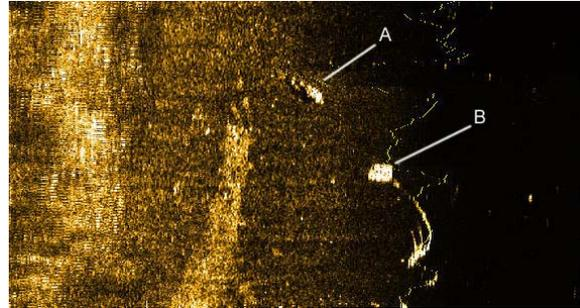
Klein 3000 Sidescan sonar image. (A) Victim's body (B) An acoustic marker dropped to mark the location .
