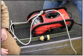
SeaBotix LBV with make-shift frame to hold lasso to retrieve drowning victim. Photo Courtesy: Truckee Police Department
