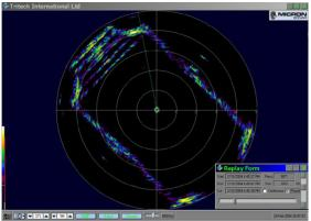
Imaging a swimming pool with a Micron Scanning Sonar.
