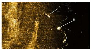
Klein 3000 Sidescan sonar image. (A) Victim's body (B) An acoustic marker dropped to mark the location . Image Courtesy: Victoria Police Underwater Security Team
