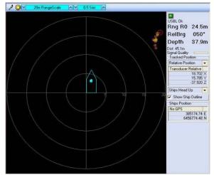
Tritech Micron Nav Tracking System software display.
