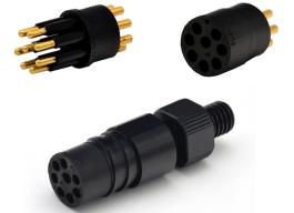
Baromax Underwater Connector series is the smallest high power density underwater connector rated for continuous submersion up to 10,000 psi. Wire sizes up to #18 AWG offers power capabilities up to 20 amps per contact. User configurable assemblies provide limitless configurations with one connector face.
