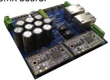
Now adding an additional IP Camera, multibeam sonar or other Ethernet based devices to small UUVs (unmanned underwater vehicles) has a "drop-in" solution. The DEPS (Dual Ethernet Plus Serial) Multiplexer is an economical approach to expanding the communication capabilities of small UUVs without major design revisions. The DEPS MUX 2.0 not only combines two Ethernet signals onto a single twisted pair (2 conductors), it can power the devices via its onboard 12VDC and 24VDC clean power supplies.
