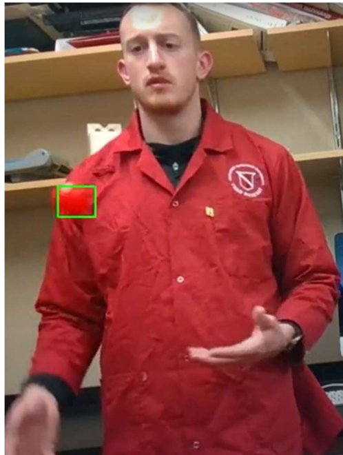
Figure 32 - Ball Detection with Same Colored Background
