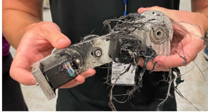
Figure 28 - Robotic Arm Recovered From Parachute
