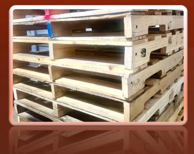
A grade a Premium is a recycled pallet where the pallet hasn't had any significant damage to it. It only had few minor repairs keeping the same standard as a brand-new pallet. It will have some color variation and a mixture of four-inch and six-inch decking. This type of pallet are mostly used by food, pharmaceutical or other industries
