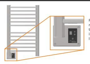
For left side electrical requests, the orientation of the DHC does not change, it is simply moved to the lower left side of the unit.
