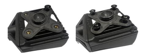
Once all fixings are loosely assembled, all 4 fixings can be fully tightened using the 3mm hey key. A criss-cross tightening pattern is recommended. Do not overtighten. Do not use power tools.
