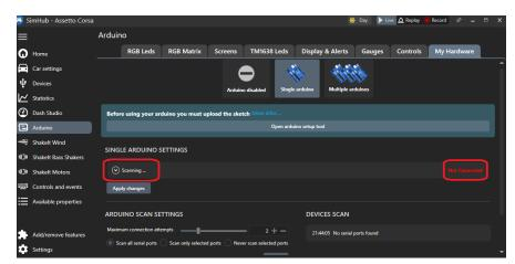
Wait approximately 30 seconds for SimHub to find the FDU device. The scanning status will change from 'Not Connected' to 'Connected' and show 'Castlespeed FDU' as the device name.
