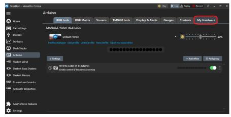
Underneath the 'arduino settings' section, you will see the SimHub software 'scanning' for new devices.
