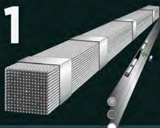
1 Spent or used fuel (incorrectly referred to as nuclear waste) is a solid – made up of ceramic **pellets** and **metal fuel rods**.
