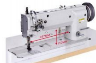
操作空间(operate space): 6610-381/6620-381: 380mmX125mm; 6610-457/6620-457: 457mmX150mm; 6610-625/6620-625: 635mmX150mm; 6610-800/6620-800: 800mmX125mm; 6610-1000/6620-1000: 1000mmX125mm
