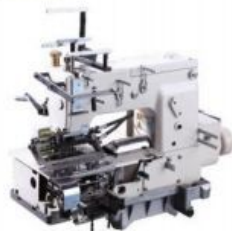
12 needle Flatbed double chainstitch for simultaneous shirring 十二针上下普通线中间橡筋线褶皱机
