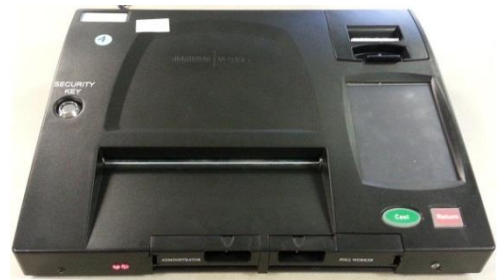
Figure 1. ImageCast Precinct tabulator (ICP)
