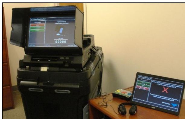
Figure 3. ICE with external, "dual" monitor
