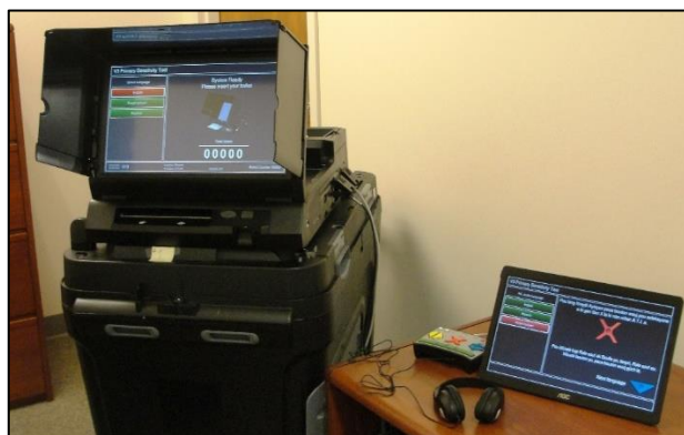
Figure 3. ICE with external, "dual" monitor
