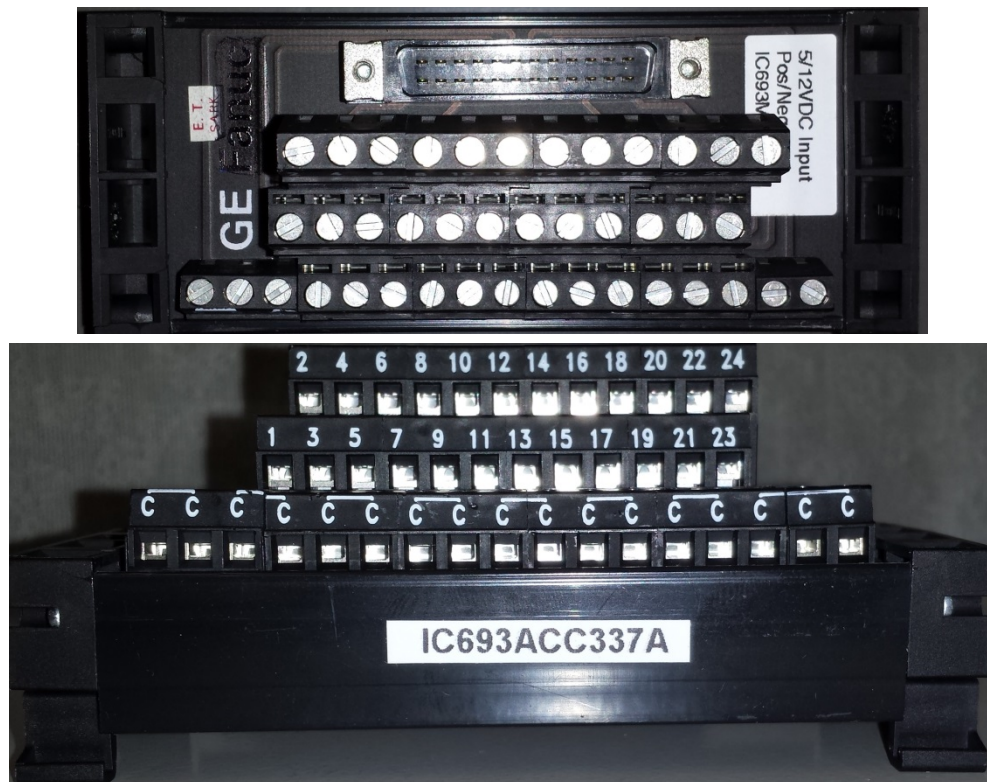
Figure 441: IC693ACC337 Terminal Block Top and Front Views
