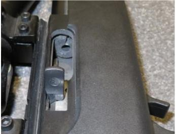
• Charging the magazine: A 0.22 Rimfire round can only be inserted into the magazine one way. The Magazine has an enlarged opening at the top. This allows the larger part of the 0.22 cartridge to be inserted, pushed down & pushed back at the same time.
