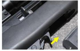
• Ruger working parts: upon firing the last shot the working parts will remain forward.
