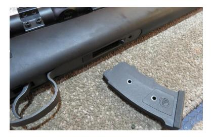
• Releasing the magazine: either magazine can be released by pulling the magazine release toward the back of the rifle, this allows the magazine to drop away.
