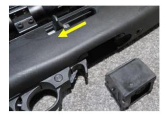
3, push the Working parts retainer back and up, hold this in place while you release the working parts
