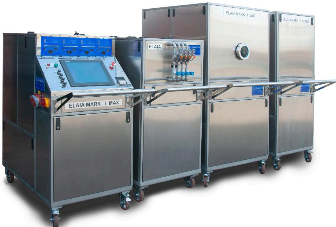
**ELAIA MARK-1 MAX system** allows cost-effectively maintain the required cleanliness of industrial and hydraulic oils in the equipment and hydraulic systems of industrial equipment, as well as prevent industrial emergencies in advance.
