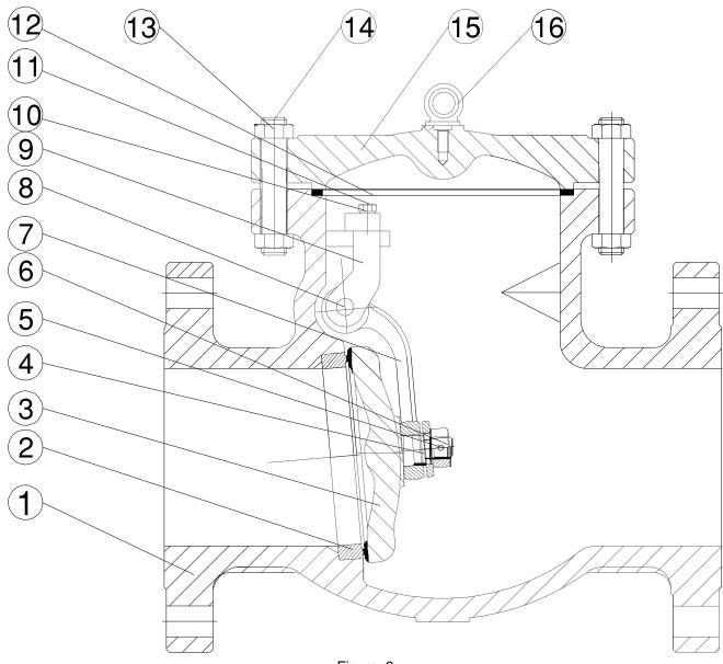
General Construction Drawing - Swing Check Valve
